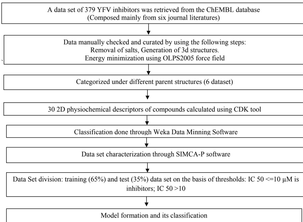
**The workflow of KNIME Based Classification [9] Models for Yellow Fever Virus Inhibition**
