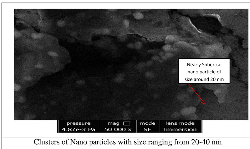
Pic No. 2: SEM images of synthesized Nanoparticles
