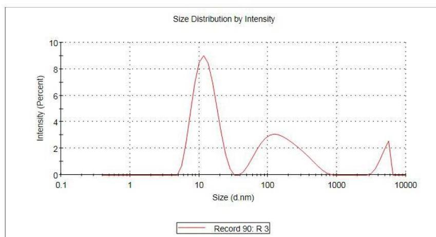
Figure2: Particles size distribution for synthesized AgNPs
